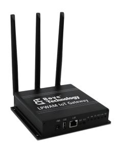
Walrus LoRaWAN-ID Gateway is an indoor IoT gateway based on LoRaWAN and targets to LPWAN network. The GW could support LoRaWAN Class A/C protocol and Wi-Fi IEEE 802.11b/g/n standard.
