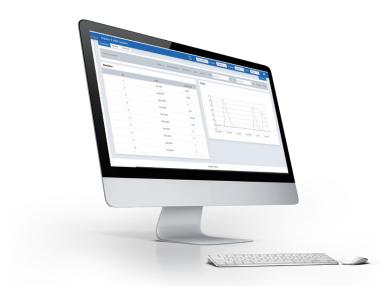
Alpaca-E AMI System is a smart metering platform for meter data collecting, remote valve controlling, visualization, and device management. It enables meter connectivity via diverse communications – LoRaWAN, NB-IoT, GPRS, etc.
